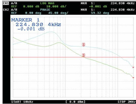
Conditions: VIN = 3.6 V, VOUT = 1.8 V, I<sub>OUT</sub> = 1.6 A; bandwidth: 224 kHz, phase margin: 59°
